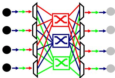
Figure 3. An AAPN star viewed as a distributed three-stage Clos switch.
