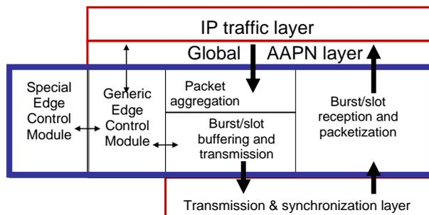
Figure 4. Edge node architecture for the prototype.
